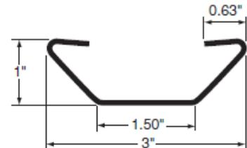
ROOF BOW, ANTI-SNAG, STEEL, 99"
